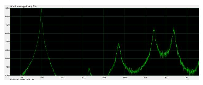
$3S \ \ \ \ Fa \ = \ \ 200 \ \ Hz \ \ audio \ peak \ filter \ \ \ Lt \ = \ \ 914 mm \qquad \qquad \ \ Vert. 5 \ db \ \ Horiz. \ 100 \ Hz$
