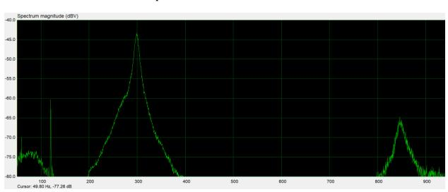
$3S \quad Fa = 350 \text{ Hz} \text{ audio peak filter } Lt = 520 \text{ mm} \qquad \text{Vert. 5 db Horiz. 100 Hz}$
